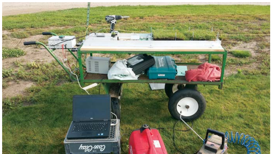
The sod tensile strength testing apparatus and data acquisition system is shown here at the St. Paul site. Photo courtesy of Joshua Friell, PhD
