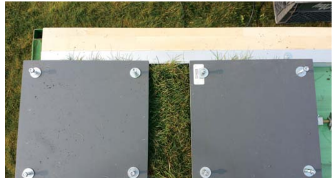
The sod tensile strength testing apparatus shown here contains a sod sample prior to testing at the St. Paul site. Photo courtesy of Joshua Friell, PhD
