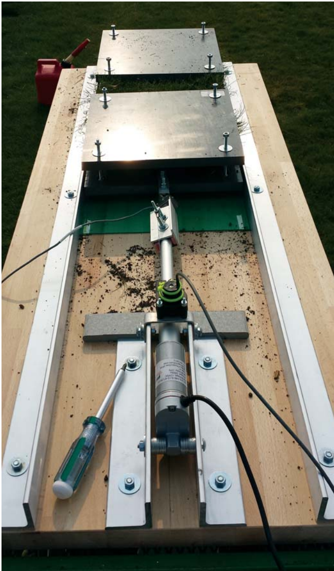
This view of the sod tensile strength testing apparatus shows the linear actuator, string potentiometer, load cell, and clamping system. Photo courtesy of Joshua Friell, PhD
