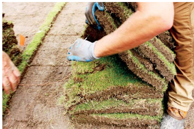
A thermocouple is being installed within this stack of sod to measure the internal temperature.
